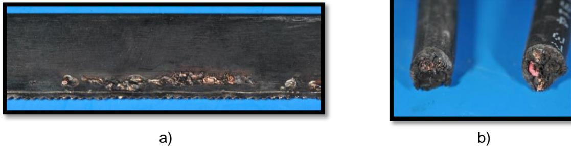
Figure 24: a) The hacksaw used in the cutting simulations after the experiments were performed and b) 1 of 5 cable samples used in the experiments after execution
